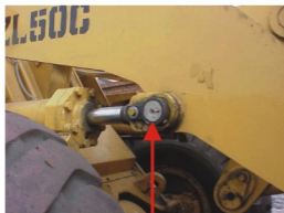
Loadcells installed here
